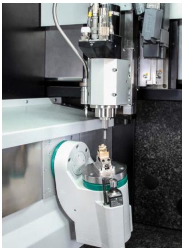
Spreitzer centre vice MZE50-20 on small 5-axes machine
