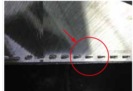
Formschlüssiges Spannen Form-closed clamping
